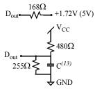
Figure B: Output load
