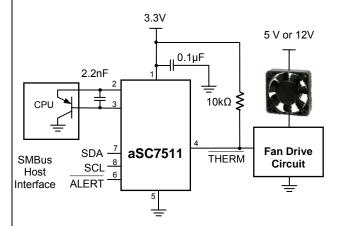
Figure 12. Simple Fan Control
