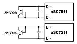
Figure 10. Discrete Remote Diode Connection
