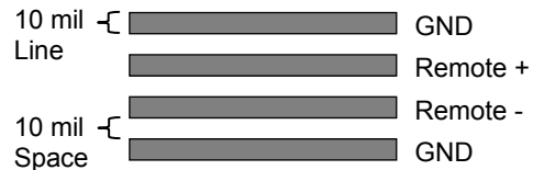
Figure 15 Recommended Remote Diode Circuit Board Interconnect
