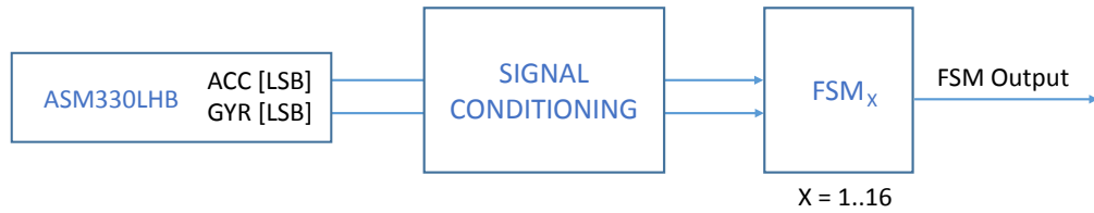
Figure 2. State machine in the ASM330LHB
