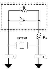
$$\label{eq:C_L} \begin{split} C_L &= 2^*(C_P - C_S), \\ Where \ C_P &= Load \ capacitance \ of \ crystal \end{split}$$
