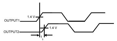
Input - Output Propagation Delay
