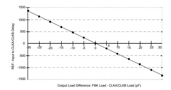
To close the feedback loop of the ASM5P2308A, the FBK pin can be driven from any of the eight available output pins. The output driving the FBK pin will be driving a total load of 7pF plus any additional load that it drives. The relative loading of this output (with respect to the remaining outputs) can adjust the input output delay. This is shown in the above graph.
