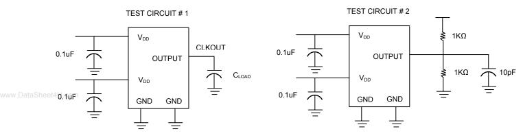
For parameter  $t_8$  (output skew rate) on -1H devices
