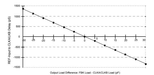
To close the feedback loop of the ASM5P23S08A, the FBK pin can be driven from any of the eight available output pins. The output driving the FBK pin will be driving a total load of 7pF plus any additional load that it drives. The relative loading of this output (with respect to the remaining outputs) can adjust the input output delay. This is shown in the above graph.
