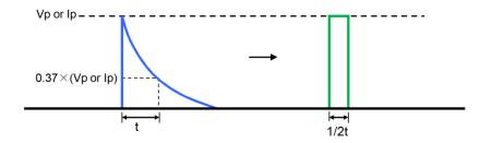
2. Damping oscillation wave with time constant of envelope "t" → Square wave
