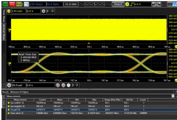
Figure 9, PCIe3.0 Eye diagram test, 8Gbps, Vpp=1V, No Device through Path
