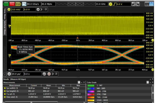
Figure 14, PCIe4.0 Eye diagram test, 16Gbps, Vpp=1.3V, No Device through Path
