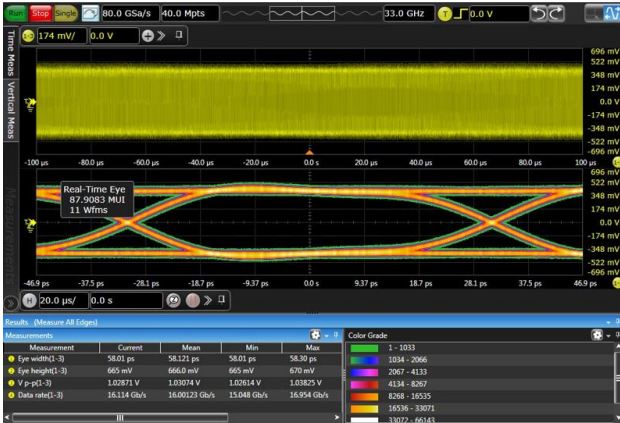
Figure 13, PCIe4.0 Eye diagram test, 16Gbps, Vpp=1V, No Device through Path
