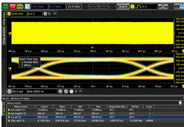
Figure 11, PCIe3.0 Eye diagram test, 8Gbps, Vpp=1V, With Device
