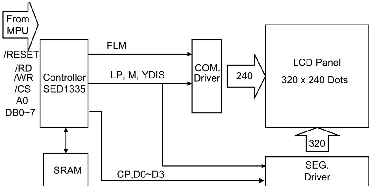
\* Please use the YDIS pin and the inner command of the SED1335 to control Display On/Off.
