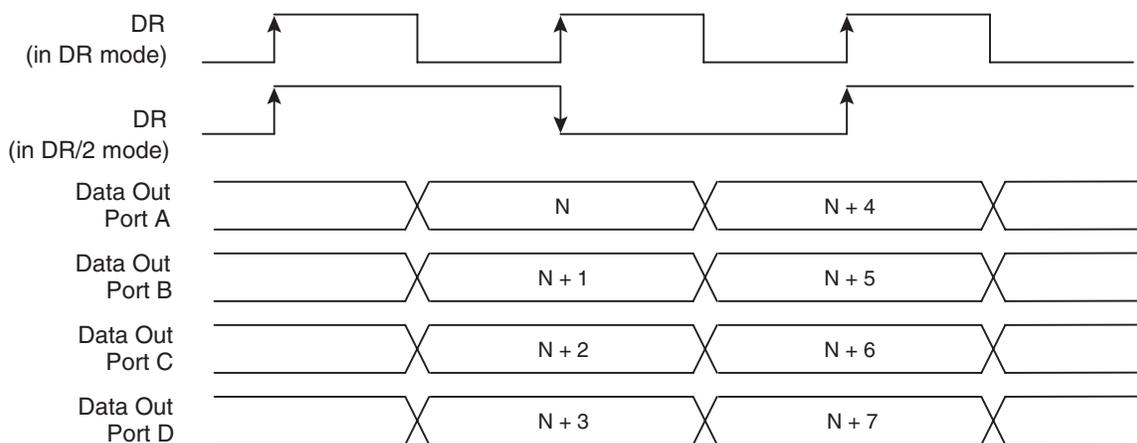
**Figure 3-8.** Staggered Mode in 1:2 Ratio (STAGG = 0)
