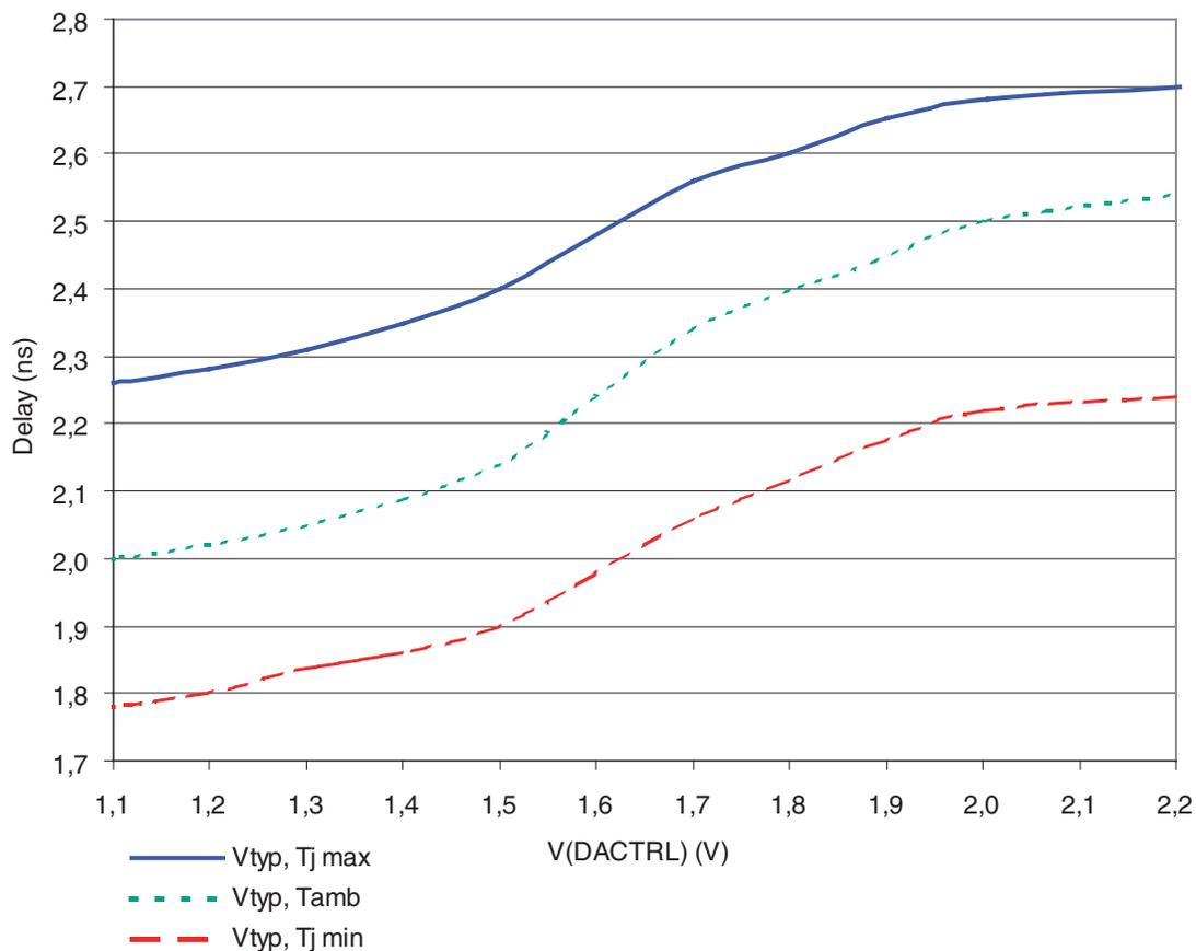
The tuning range is not constant over the specified temperature range. The longest tuning range is obtained in typical conditions (typical power supplies and ambient temperature) and it slightly decreases when temperature is rising or decreasing.
