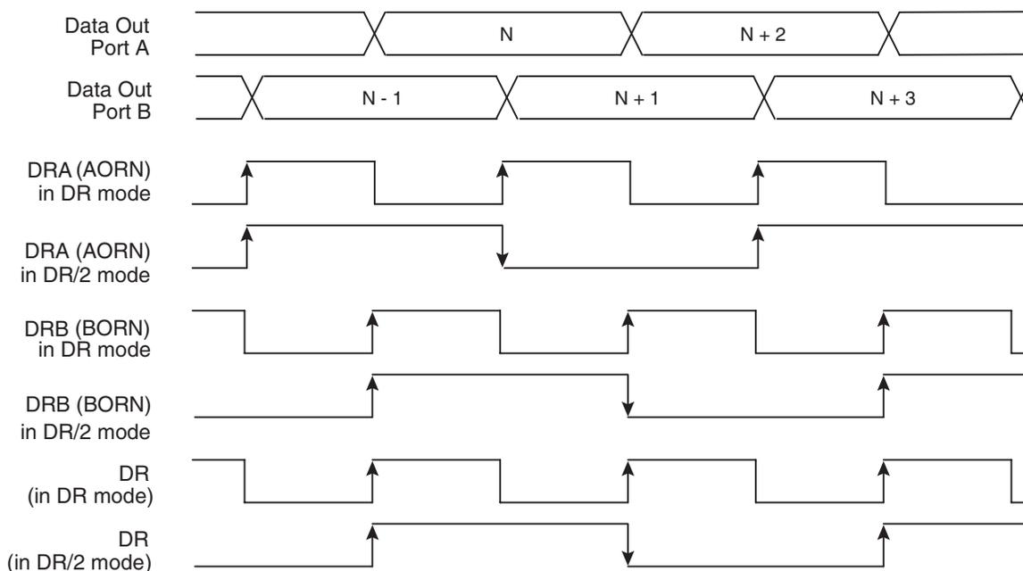
**Figure 3-9.** Staggered Mode in 1:4 Ratio (STAGG = 0)
