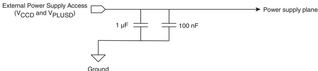
Each group of neighboring power supply pins attributed to the same value should be bypassed with at least one pair of 100 pF capacitors in parallel to 10 nF capacitors. These capacitors should be placed as close as possible to the power supply package pins.
