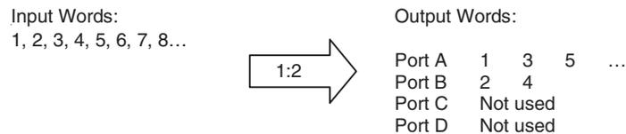
Note: Ports C & D data have undetermined level. They can be left unconnected.
