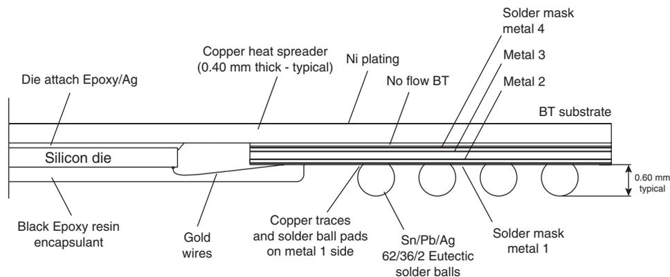
Note: In the DMUX package above, the die's underside is attached to the copper heat spreader so the copper heat spreader is at GND (0V). We recommend electrically isolating the copper heat spreader from the heat sink if a heat sink is used, in which case adequate low Rth electrical isolation should be used.
