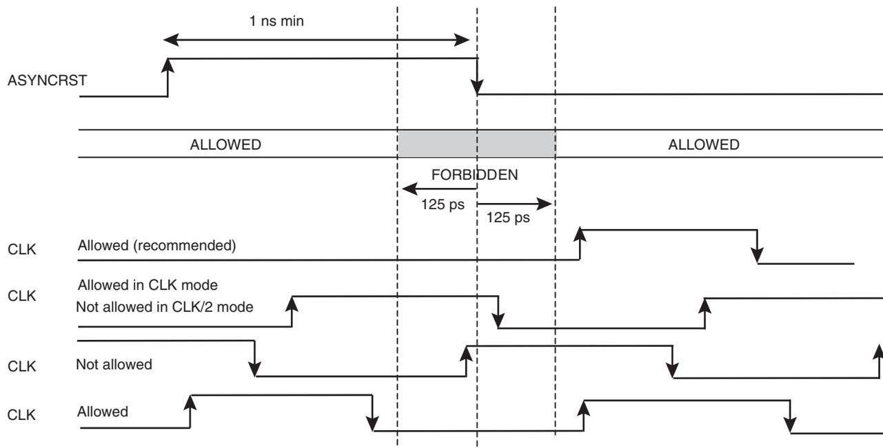
It is highly recommended to stop the clock at the Low level when ASYNCRST is active (high level). Note that when e2v's ADCs are in reset, the ADC Data Ready output (input clock of the DMUX) is stopped at the low level. In the case where the clock can not be stopped during the reset (not recommended), it is not allowed to have an active edge (rising edge in CLK mode but both rising and falling edge in CLK/2 mode) of the CLK clock within a  $\pm 125$  ps area around the falling edge of ASYNCRST.
