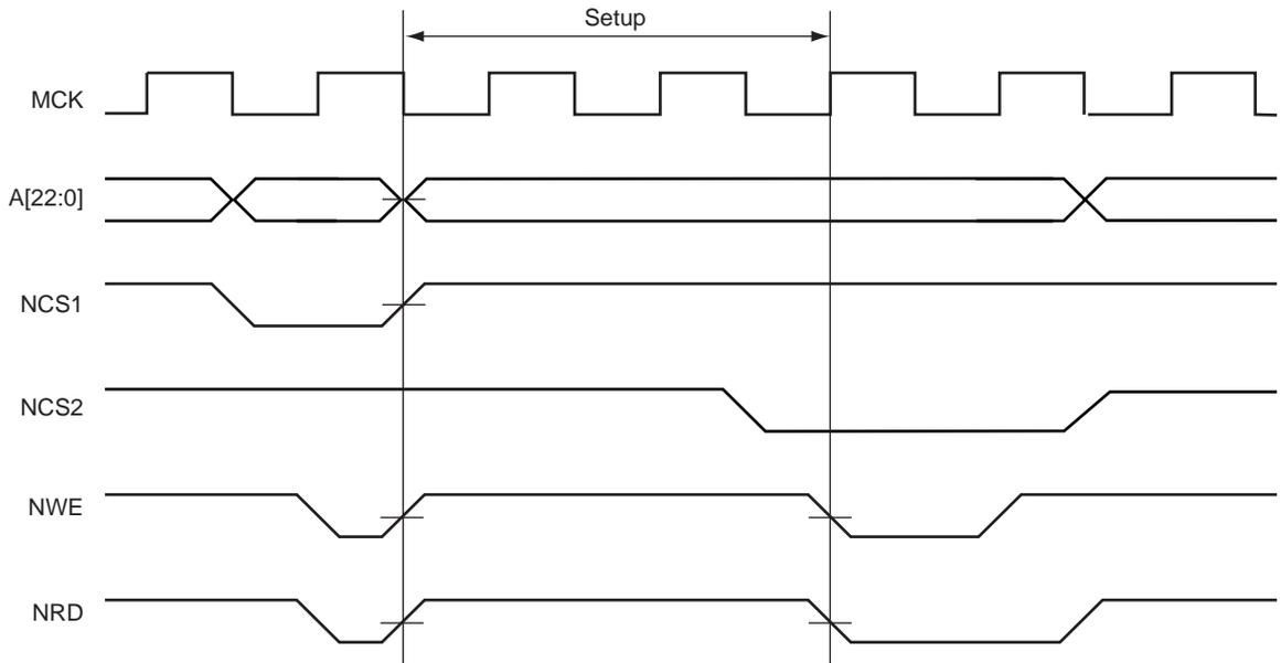
**Figure 17-24. First Access with Data Float Wait States (TDF = 2) and Second Access with Setup (NRDSETUP = 1)**
