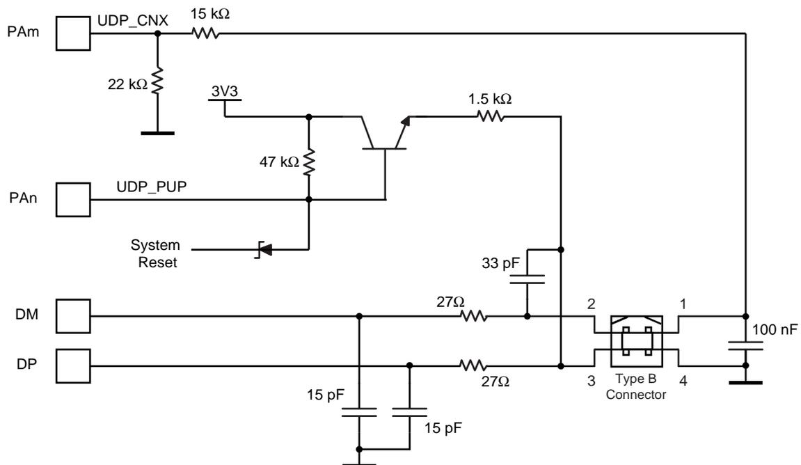
UDP\_CNX is an input signal used to check if the host is connected
