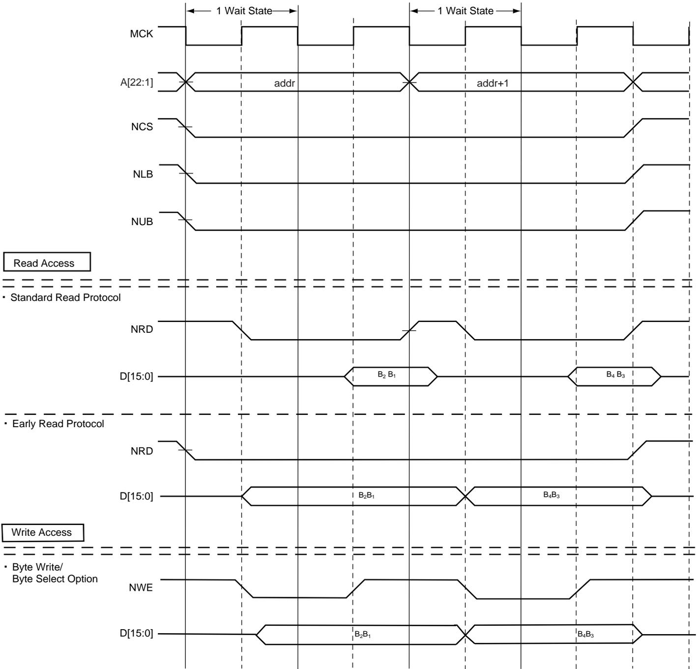
Figure 17-40. 1 Wait State, 16-bit Bus Width, Half-Word Transfer
