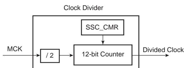
The Master Clock divider is determined by the 12-bit field DIV counter and comparator (so its maximal value is 4095) in the Clock Mode Register SSC\_CM, allowing a Master Clock division by up to 8190. The Divided Clock is provided to both the Receiver and Transmitter. When this field is programmed to 0, the Clock Divider is not used and remains inactive.
