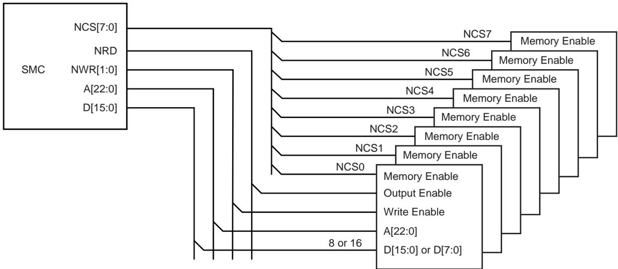
Note: 1. The maximum address space per device is 8 Mbytes.
