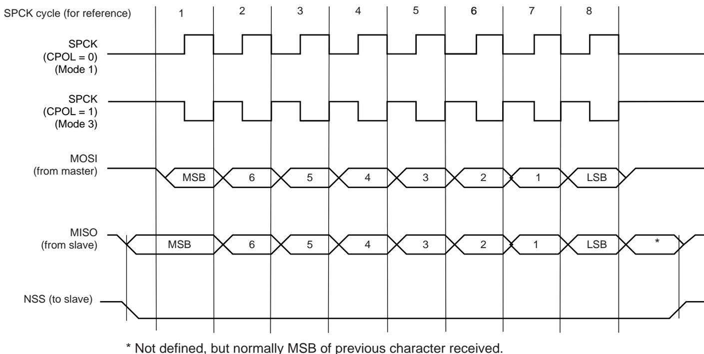
**Figure 27-8. SPI Transfer Format (NCPHA = 0, 8 bits per transfer)**
