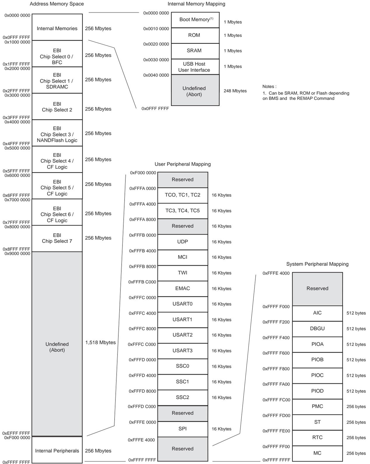
A first level of address decoding is performed by the Memory Controller, i.e., by the implementation of the Advanced System Bus (ASB) with additional features.
