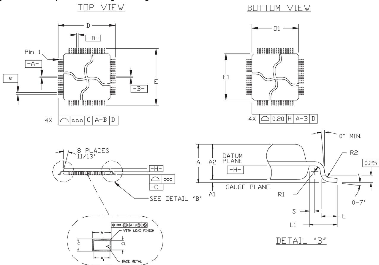
Table 38-3. 208-pin PQFP Package Dimensions (in mm)
