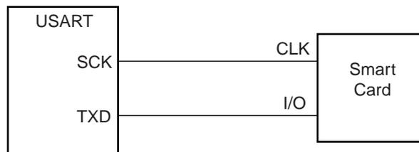
When operating in ISO7816, either in T = 0 or T = 1 modes, the character format is fixed. The configuration is 8 data bits, even parity and 1 or 2 stop bits, regardless of the values programmed in the CHRL, MODE9, PAR and CHMODE fields. MSBF can be used to transmit LSB or MSB first.
