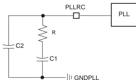
Values of R, C1 and C2 to be connected to the PLLRC pins must be calculated as a function of the PLL input frequency, the PLL output frequency and the phase margin. A trade-off has to be found between output signal overshoot and startup time.
