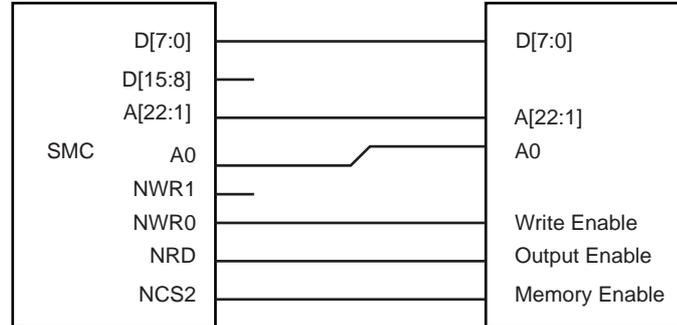
Figure 17-5 shows how to connect a 512K x 16-bit memory on NCS2 (DBW = 01).
