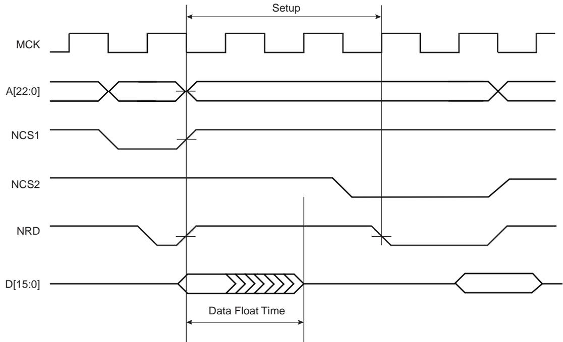
**Figure 17-25. First Access with Data Float Wait States (TDF = 2) and Second Access with Setup (NRDSETUP = 3)**
