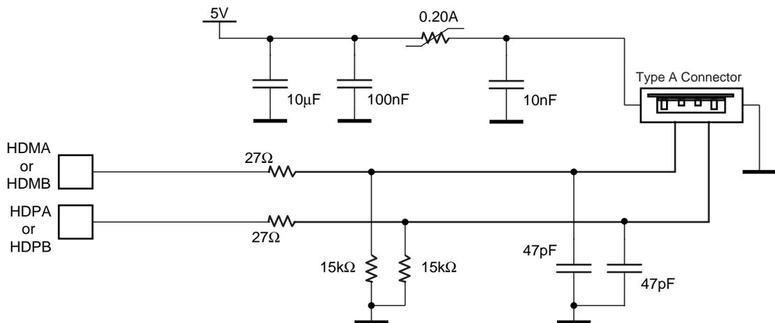
As device connection is automatically detected by the USB host port logic, a pull-down must be connected on DP and DM on the board. Otherwise the USB host will permanently detect a device connection on this port.
