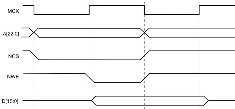
**Figure 17-10. Write Access with 1 Wait State**
