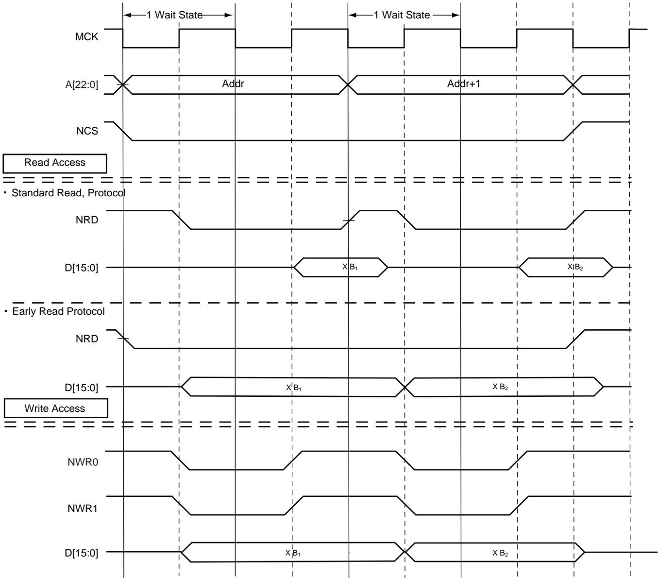
Figure 17-43. 1 Wait State, 8-bit Bus Width, Byte Transfer
