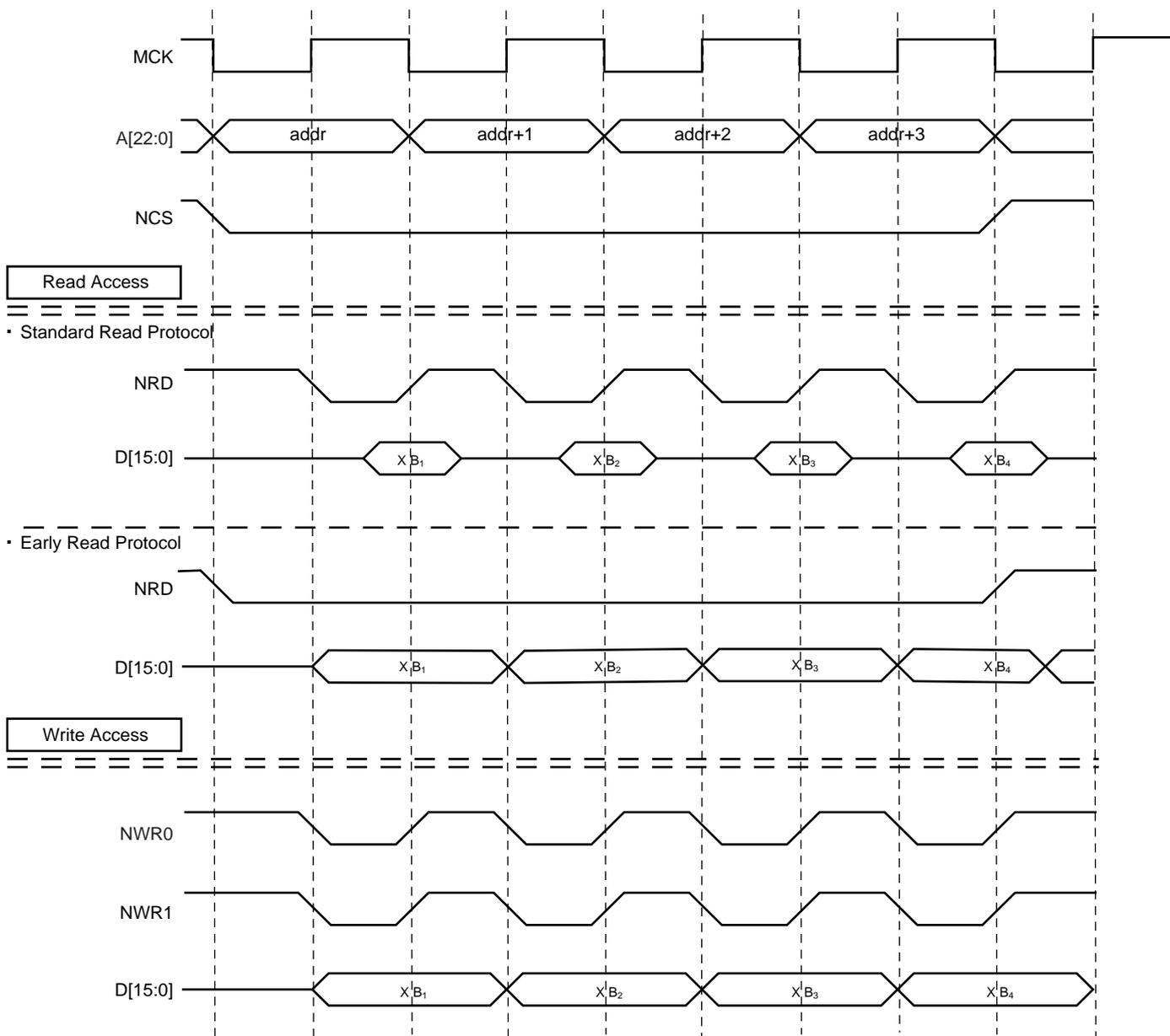
Figure 17-42. 1 Wait State, 8-bit Bus Width, Half-Word Transfer
