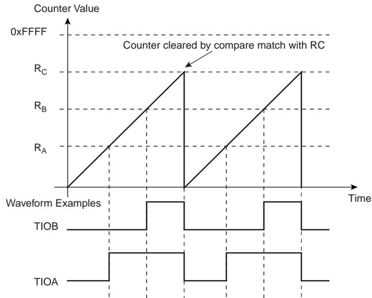
**Figure 31-9. WAVSEL = 10 With Trigger**
