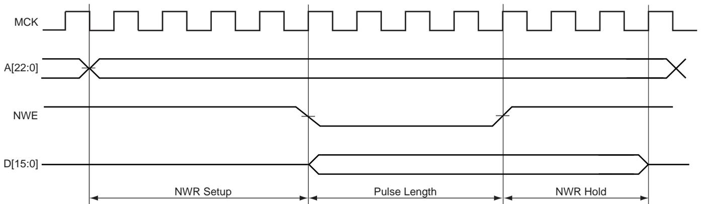
**Figure 17-22. Write Access with Setup**
