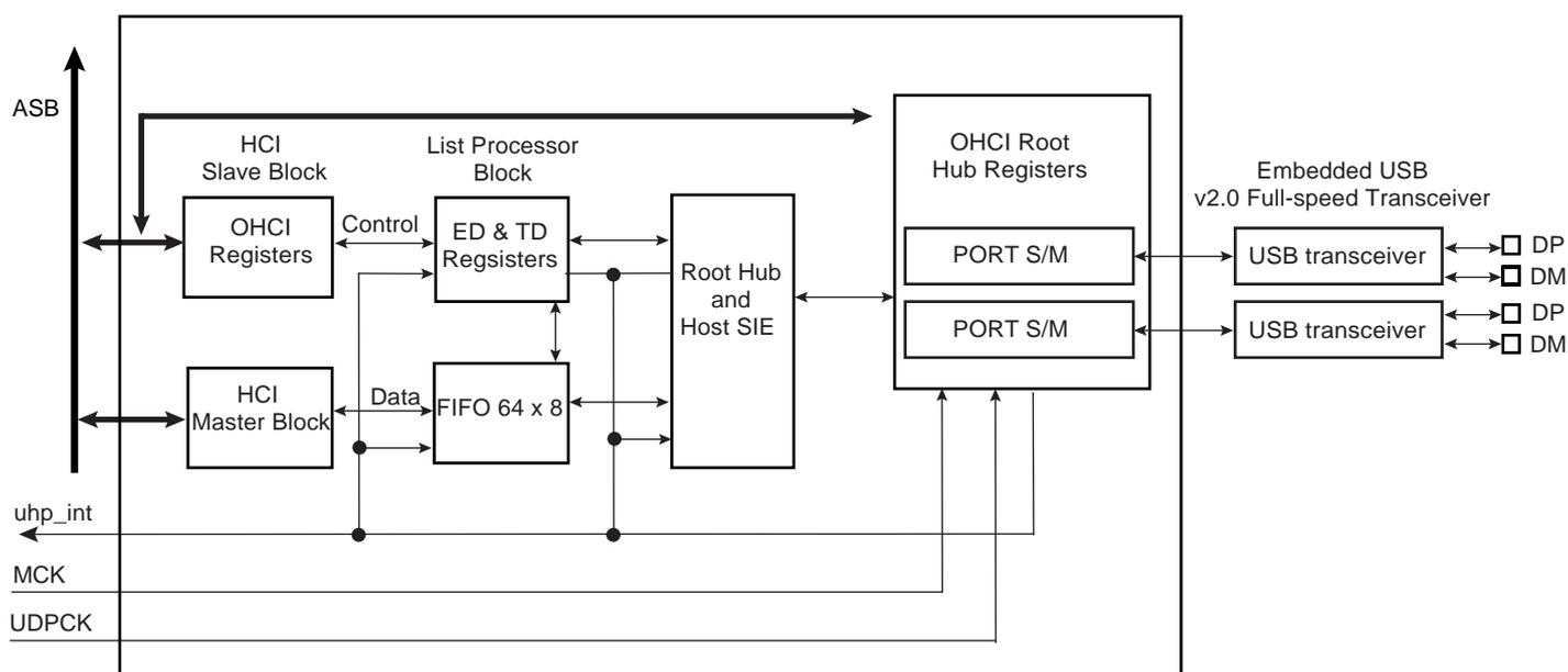
Access to the USB host operational registers is achieved through the ASB bus interface. The Open HCI host controller initializes master DMA transfers with the ASB bus as follows:
