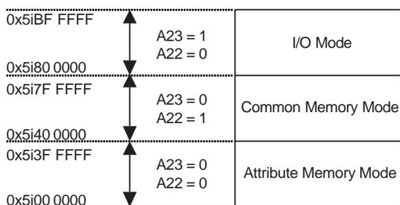
Note: In the above example, the A22 pin of the EBI can be used to drive the REG signal of the CompactFlash Device.
