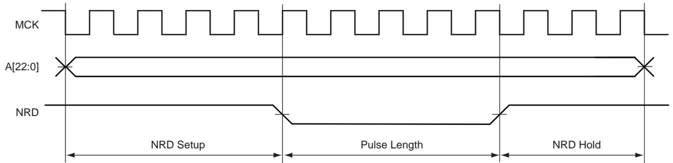
**Figure 17-20. Read Access with Setup**
