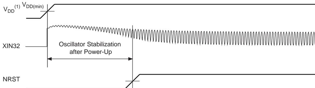
Note: 1. VDD is applicable to VDDIOM, VDDIOP, VDDPLL, VDDOSC and VDDCORE
