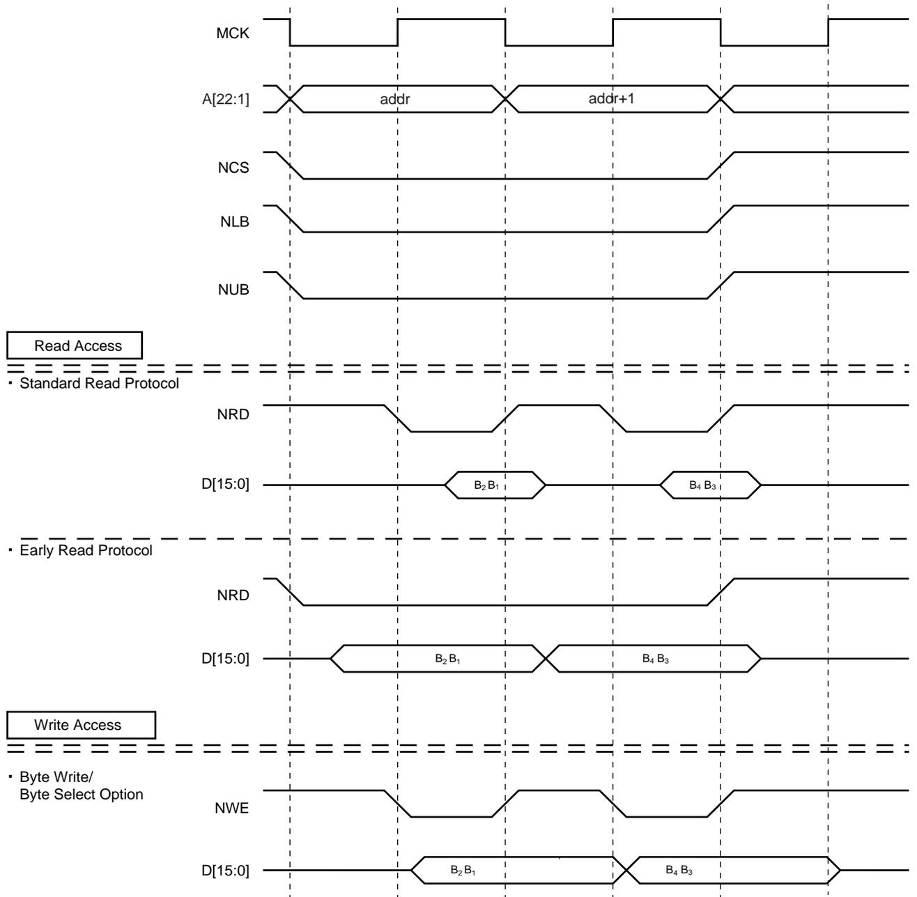
Figure 17-39. 1 Wait State, 16-bit Bus Width, Word Transfer
