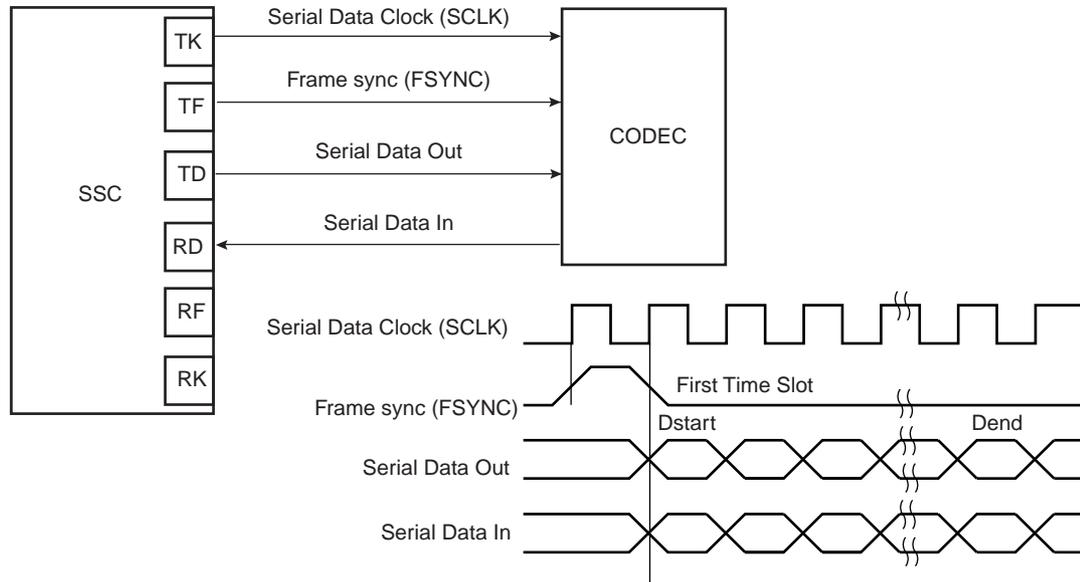
**Figure 30-18. Time Slot Application Block Diagram**
