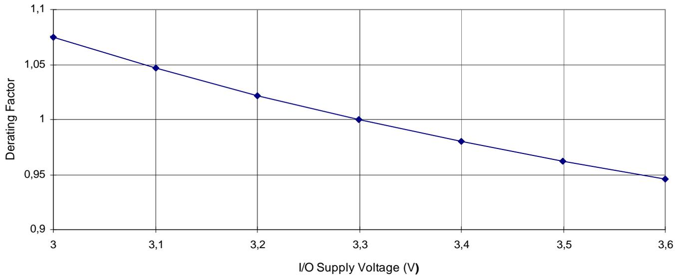
Note: The derating factor in this example is applicable only to timings related to output pins.
