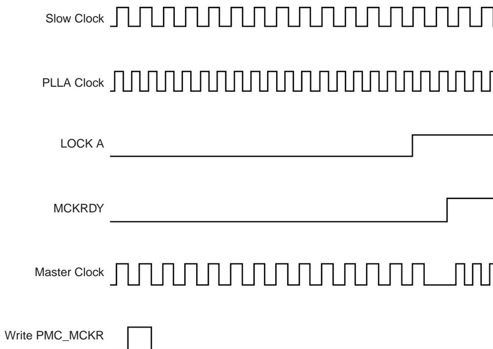
**Figure 22-10. Switch Master Clock from Main Clock to Slow Clock**
