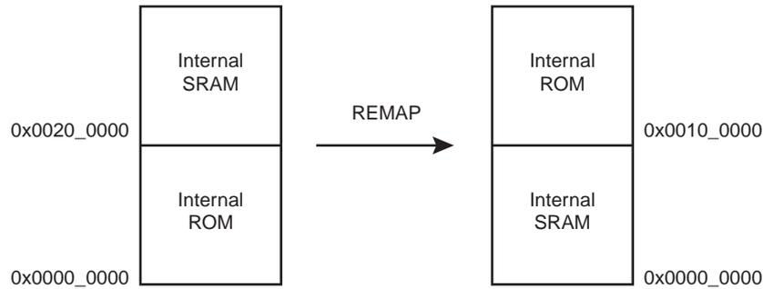
After reset, the code in internal ROM is mapped at both addresses 0x0000\_0000 and 0x0010\_0000:
