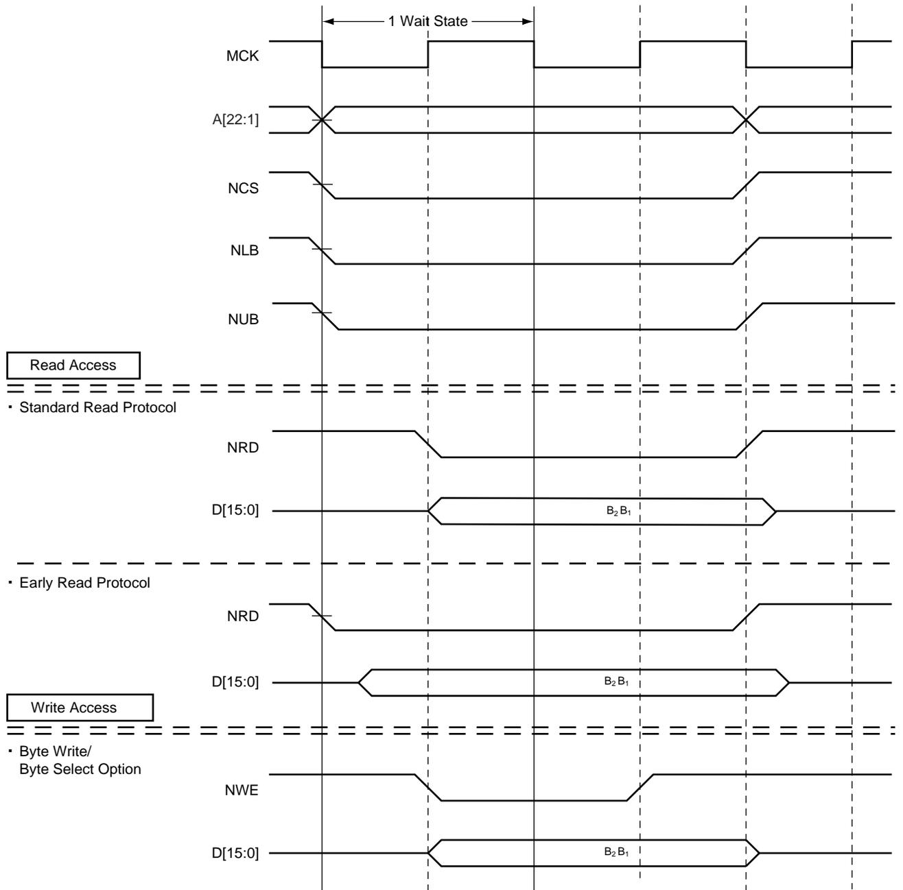
Figure 17-41. 0 Wait State, 8-bit Bus Width, Word Transfer
