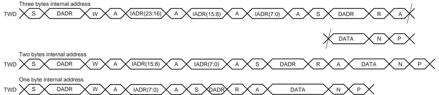
**Figure 28-8. Master Read with One Byte Internal Address and Multiple Data Bytes**
