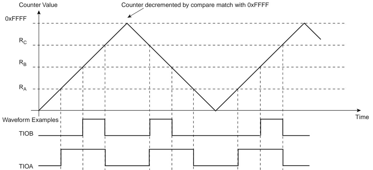
**Figure 31-11. WAVSEL = 01 With Trigger**
