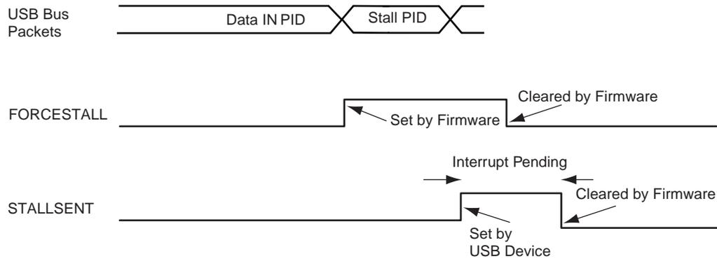
**Figure 33-15. Stall Handshake (Data OUT Transfer)**
