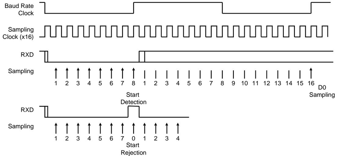
**Figure 29-8. Asynchronous Character Reception**
