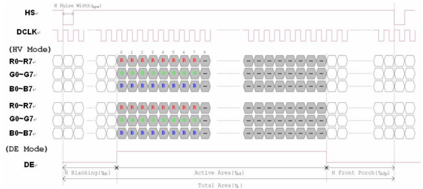
Figure 3.1 Horizontal input timing diagram.
