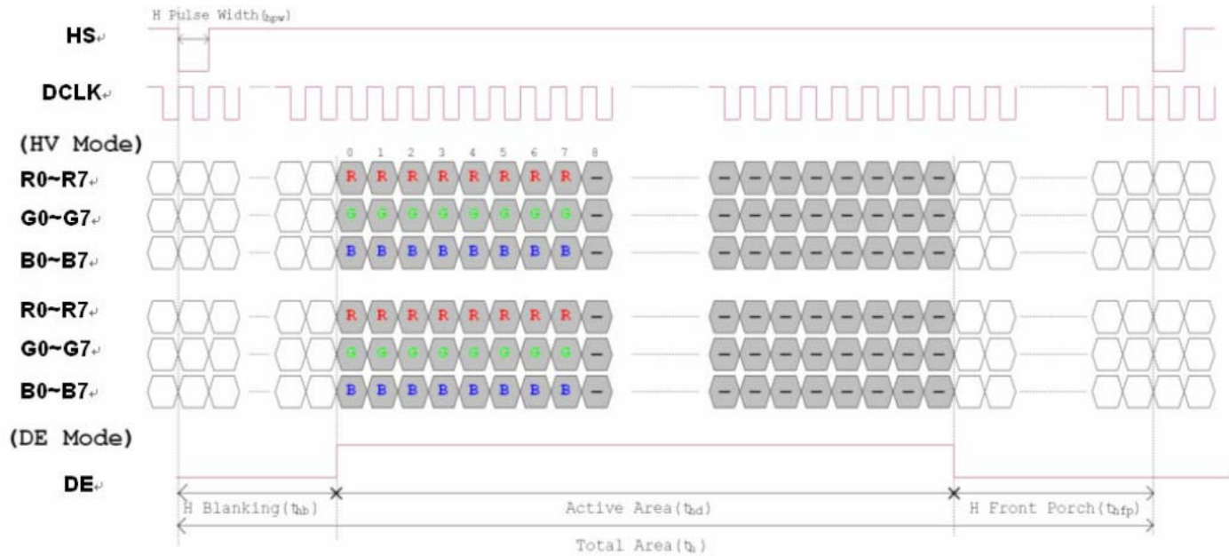
Figure 3.1 Horizontal input timing diagram.
