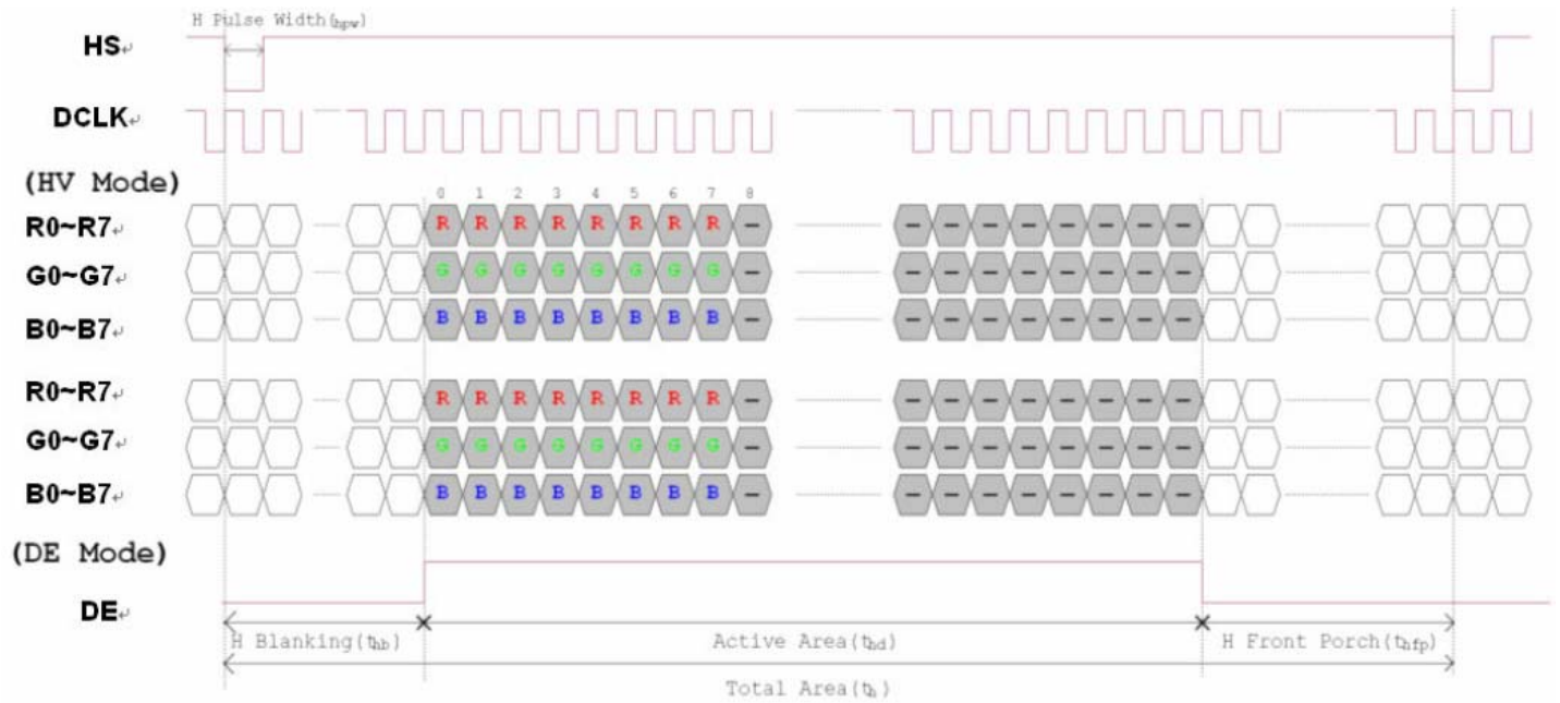
Figure 3.1 Horizontal input timing diagram.
