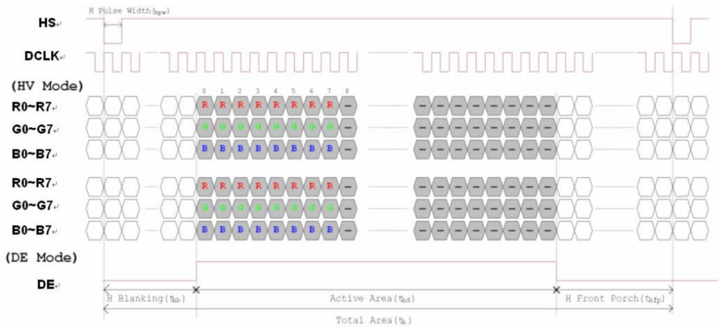
Figure 3.1 Horizontal input timing diagram.
