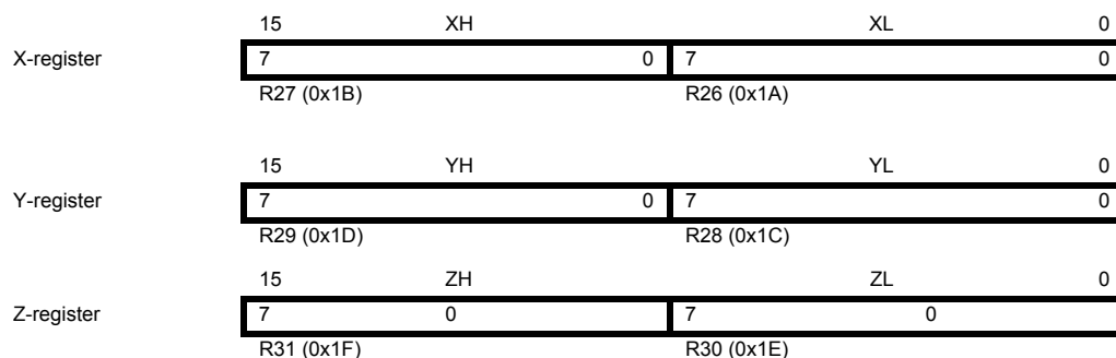
Figure 7-3. The X-, Y-, and Z-registers
