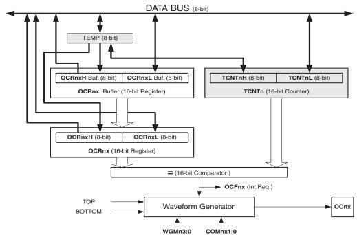
Figure 16-4. Output Compare Unit, Block Diagram
