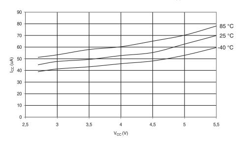
Figure 28-53. 32 kHz Tosc Current vs.  $V_{CC}$  (Watchdog Timer Disabled)
