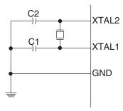
The Oscillator can operate in three different modes, each optimized for a specific frequency range. The operating mode is selected by the fuses CKSEL3:1 as shown in Table 8-3.
