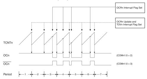
The Timer/Counter Overflow Flag (TOV0) is set each time the counter reaches MAX. If the interrupt is enabled, the interrupt handler routine can be used for updating the compare value.
