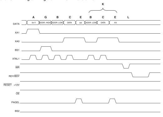
Figure 26-4. Programming the EEPROM Waveforms
