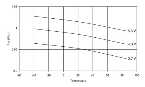
Figure 28-47. Calibrated 1 MHz RC Oscillator Frequency vs.  $V_{\rm CC}$
