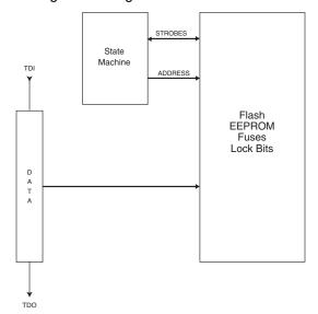
Figure 26-13. Virtual Flash Page Load Register
