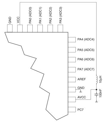
Figure 22-9. ADC Power Connections
