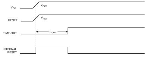
Figure 10-3. MCU Start-up, RESET Extended Externally
