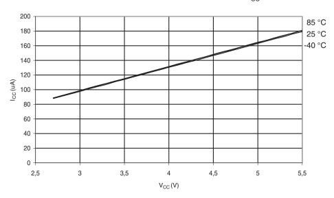
Figure 28-52. Analog Comparator Current vs.  $V_{\rm CC}$
