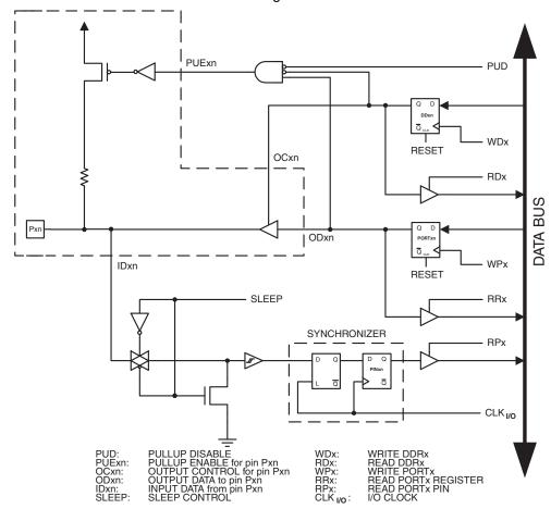
Figure 24-4. General Port Pin Schematic Diagram<sup>(1)</sup>
