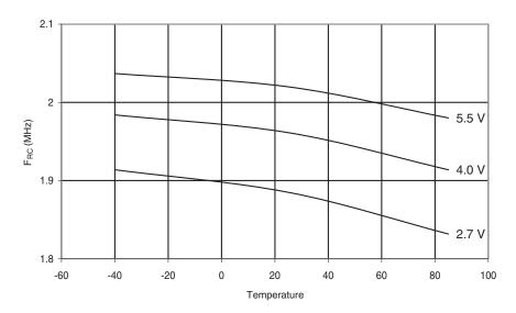
Figure 28-44. Calibrated 2 MHz RC Oscillator Frequency vs.  $V_{\rm CC}$
