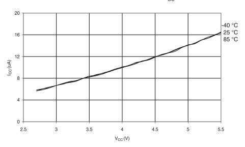
Figure 28-55. Programming Current vs.  $V_{\text{CC}}$
