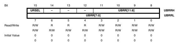
The UBRRH Register shares the same I/O location as the UCSRC Register. See the "Accessing UBRRH/ UCSRC Registers" on page 164 section which describes how to access this register.
