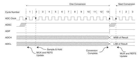
Figure 22-6. ADC Timing Diagram, Auto Triggered Conversion
