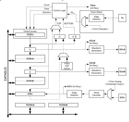
Figure 16-1. 16-bit Timer/Counter Block Diagram<sup>(1)</sup>
