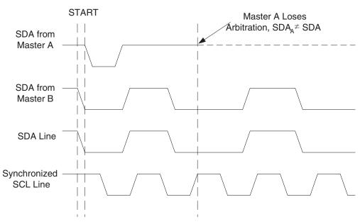
Figure 20-8. Arbitration between Two Masters
