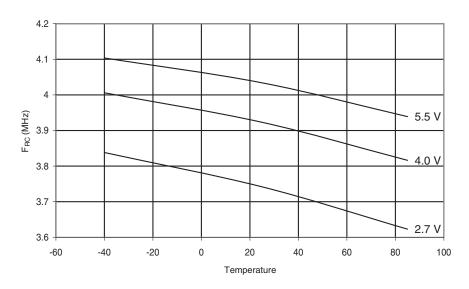
Figure 28-41. Calibrated 4 MHz RC Oscillator Frequency vs.  $V_{\rm CC}$
