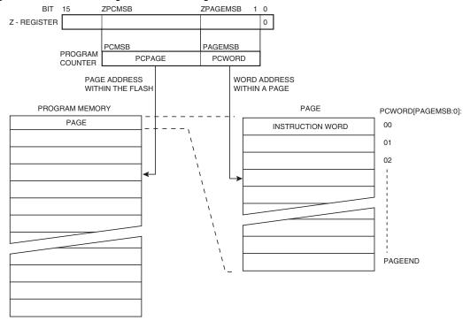
Figure 25-3. Addressing the Flash during SPM<sup>(1)</sup>
