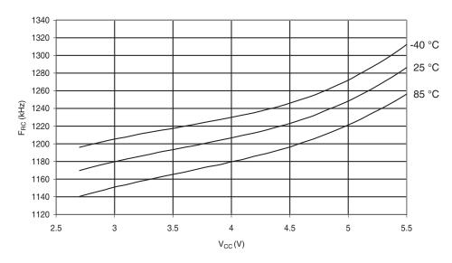
Figure 28-37. Calibrated 8 MHz RC Oscillator Frequency vs. Temperature
