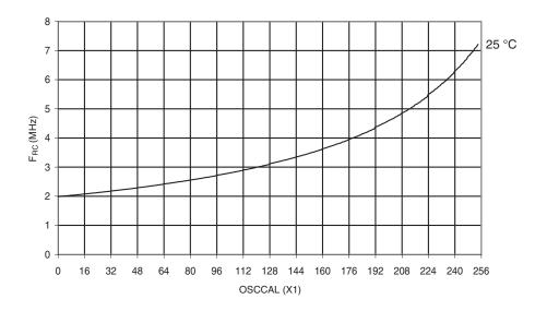
Figure 28-43. Calibrated 2 MHz RC Oscillator Frequency vs. Temperature
