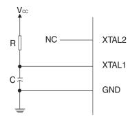
The Oscillator can operate in four different modes, each optimized for a specific frequency range. The operating mode is selected by the fuses CKSEL3:0 as shown in Table 8-6.
