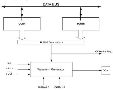
The OCR0 Register is double buffered when using any of the Pulse Width Modulation (PWM) modes. For the normal and Clear Timer on Compare (CTC) modes of operation, the double buffering is disabled. The double buffering synchronizes the update of the OCR0 Compare Register to either top or bottom of the counting sequence. The synchronization prevents the occurrence of odd-length, non-symmetrical PWM pulses, thereby making the output glitch-free.
