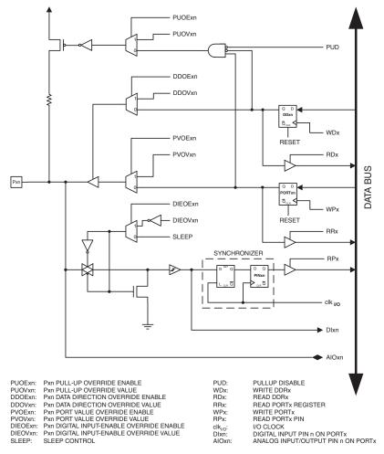
Note: 1. WPx, WDx, RRx, RPx, and RDx are common to all pins within the same port. clk<sub>I/O</sub>, SLEEP, and PUD are common to all ports. All other signals are unique for each pin.
