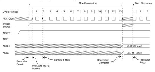
Figure 22-7. ADC Timing Diagram, Free Running Conversion
