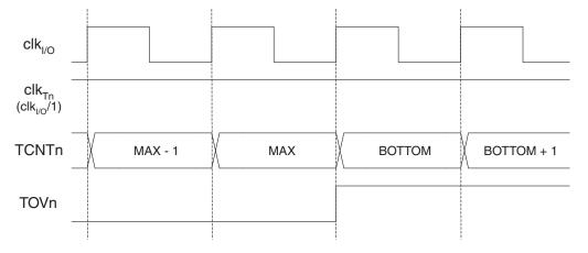
Figure 14-9 shows the same timing data, but with the prescaler enabled.
