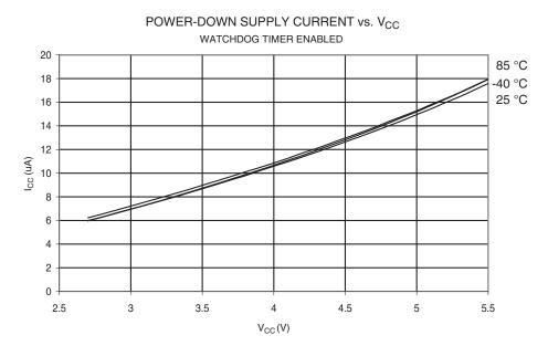
Figure 28-16. Power-Down Supply Current vs. V<sub>CC</sub> (Watchdog Timer Enabled)
