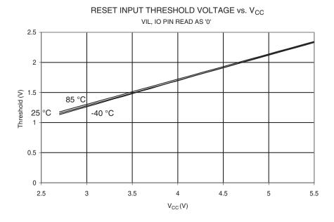
Figure 28-32. Reset Input Pin Hysteresis vs.  $V_{\rm CC}$
