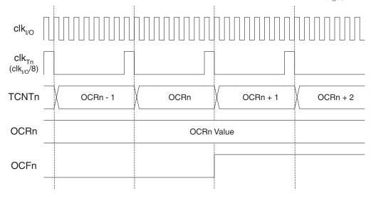
Figure 14-11 shows the setting of OCF0 and the clearing of TCNT0 in CTC mode.
