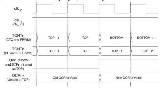
Figure 16-13 shows the same timing data, but with the prescaler enabled.
