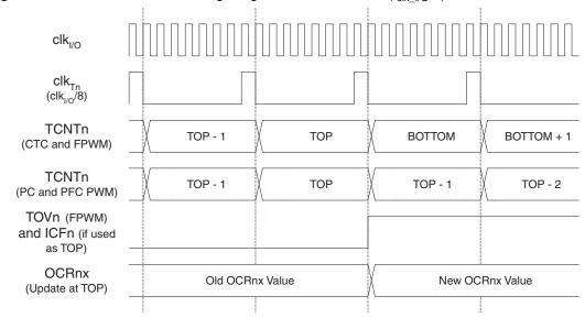
Figure 16-13. Timer/Counter Timing Diagram, with Prescaler (fclk 1/0/8)
