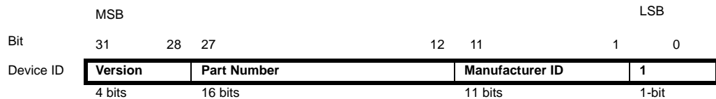
Figure 27-1. The Format of the Device Identification Register
