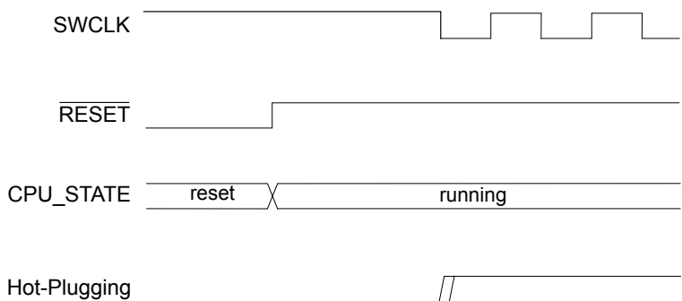
Figure 14-3. Hot-Plugging Detection Timing Diagram
