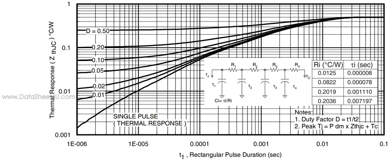
Fig 13. Maximum Effective Transient Thermal Impedance, Junction-to-Case
