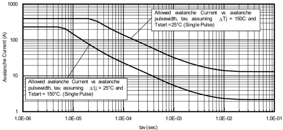
**Fig 16. Typical Avalanche Current vs. Pulse Width**
