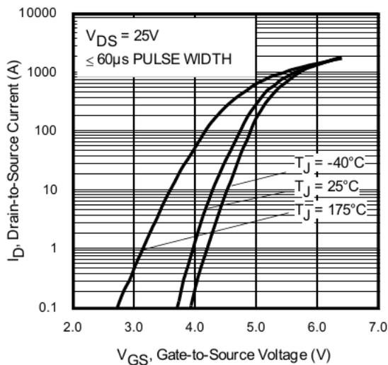
**Fig 5.** Transfer Characteristics
