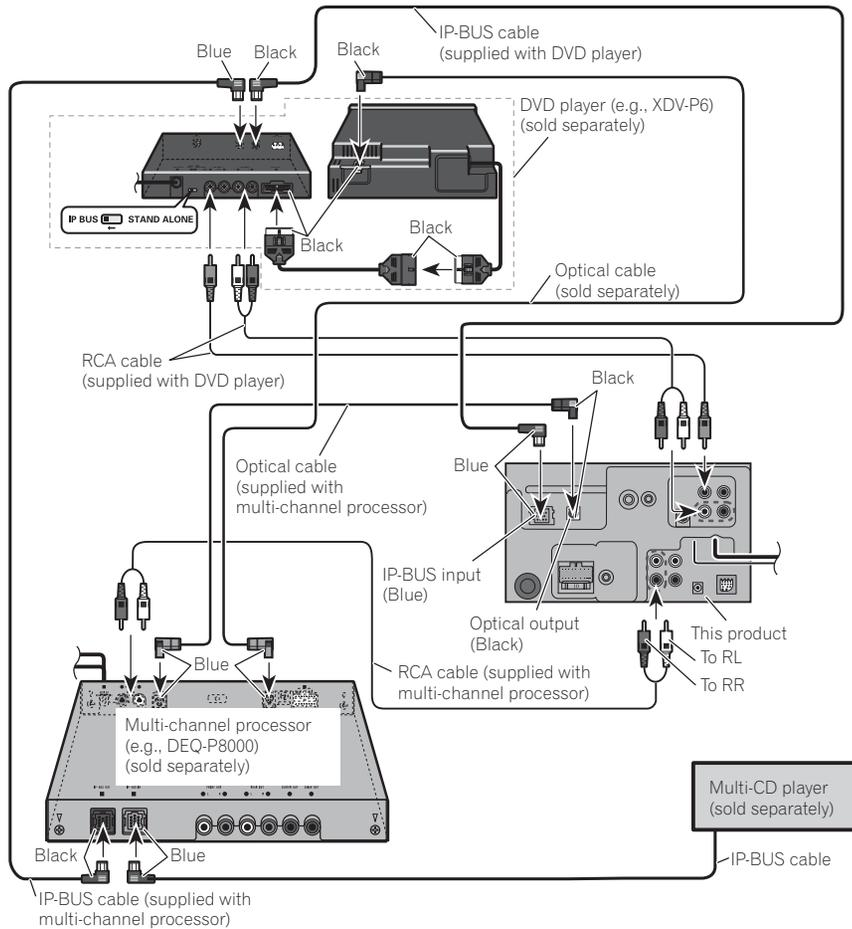
When you connect a separately sold DVD player to the separately sold multi-channel processor, the optical cable from DVD player must be connected to the optical cable 2 input (OPT. IN2) of the multi-channel processor.
