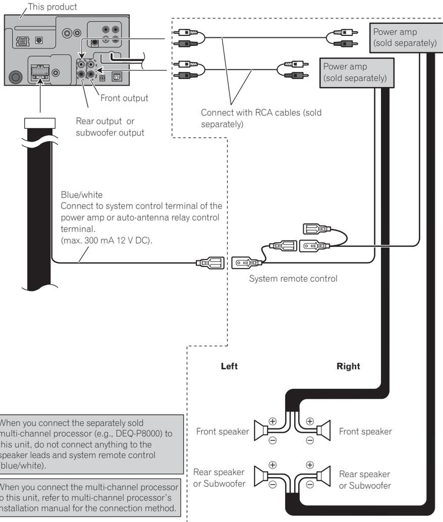
When you connect the separately sold multi-channel processor (e.g., DEQ-P8000) to this unit, do not connect anything to the speaker leads and system remote control (blue/white).
