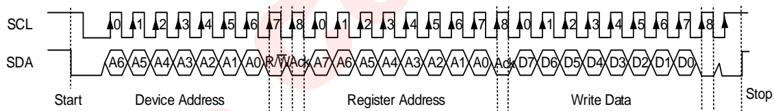
Fig 37 I 2 C Write Timing
