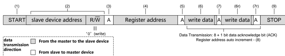
Figure 16 Writing process (data transmission direction remains the same)
