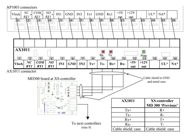
**Cable shield:** Cable shield **must** always be connected to metal case on both sides (AEpack and XS-controller).
