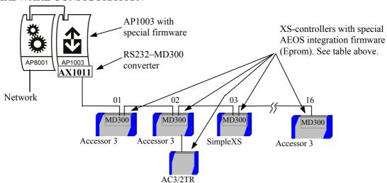
A loop of 8 XS Controllers can be controlled by a single AEpack/AEpu pair. However, keep in mind that the integrated loop becomes less decentralized compared to the original XS loop. This can partly be compensated by splitting long XS Controller loops into several small loops each controlled by separate AEpack/AEpu pairs.
