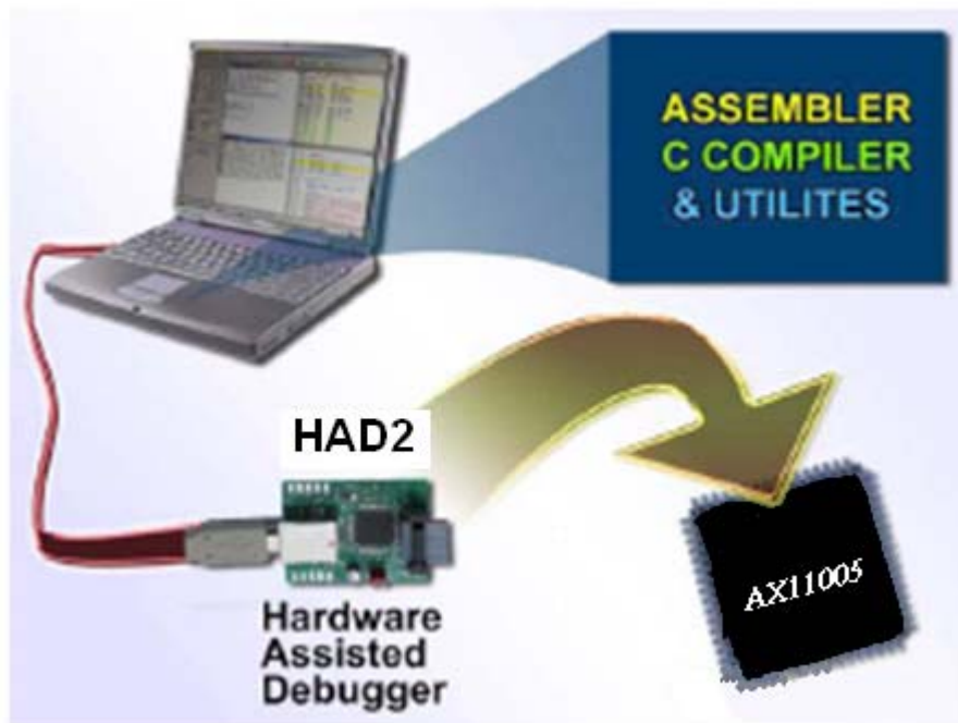
Figure 10: Typical Debugger and Hardware Assisted Debugger (HAD2) System Diagram
