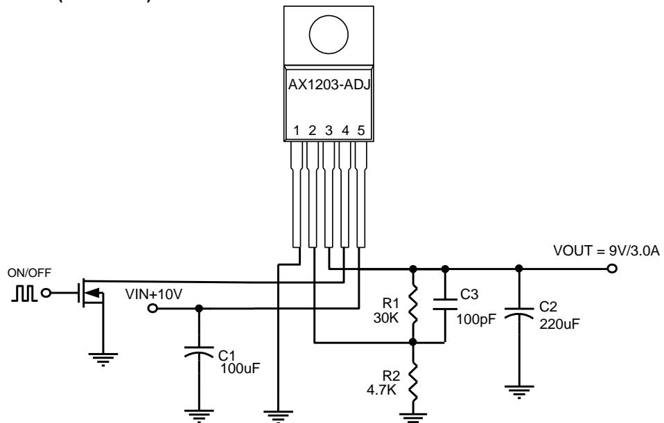
$$V_{OUT} = V_{FB} * (1 + R1/R2)$$
