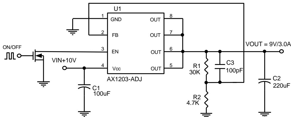
$$V_{OUT} = V_{FB} * (1 + R1/R2)$$
