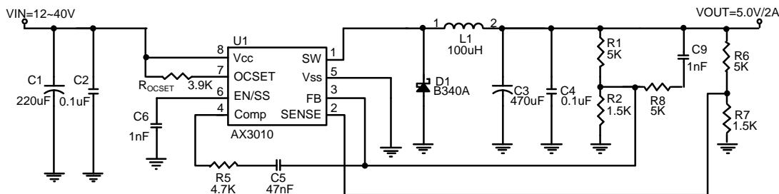
$$V_{\text{OUT}} = V_{\text{FB}} \times \left(1 + \frac{R_1}{R_2}\right), V_{\text{FB}} = 1.155V, R_2 = 0.7K \sim 1.8K$$
