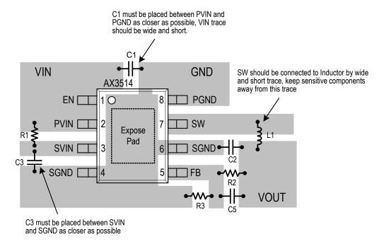
C1 must be placed between PVIN and PGND as closer as possible, VIN trace should be wide and short.
