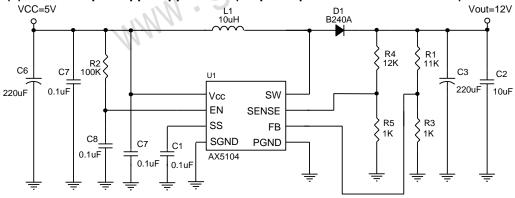
$$V_{OUT} = V_{FB} \times (1 + \frac{R1}{R3}), V_{FB} = 1.0V, R3 = 1K \sim 3K\Omega$$
