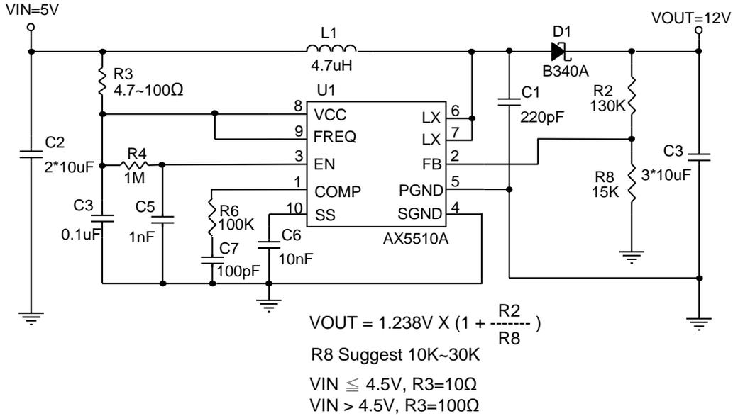
(2) FREQ=Low (Frequency=680KHz) (MSOP-10L and TDFN-10L)
