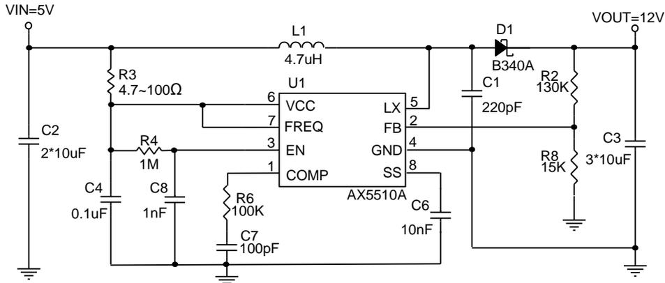
$$V_{OUT} = 1.238V \times \left(1 + \frac{R2}{R8}\right)$$
