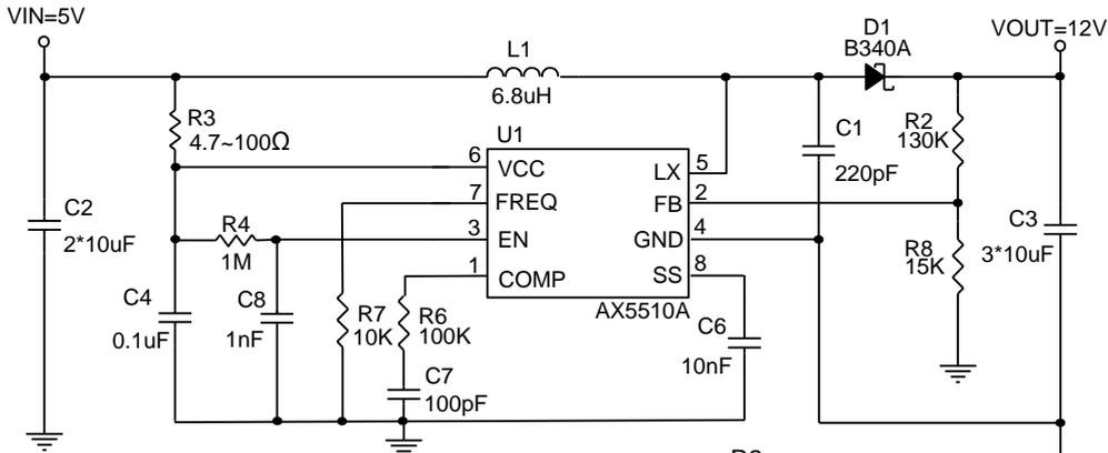
$$V_{OUT} = 1.238V \times \left(1 + \frac{R2}{R8}\right)$$
