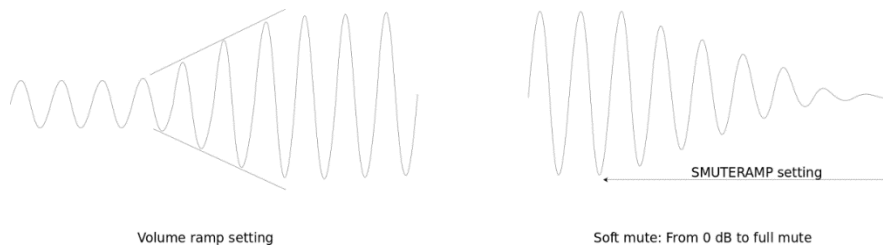
Figure 31. Volume control behavior in waveforms
