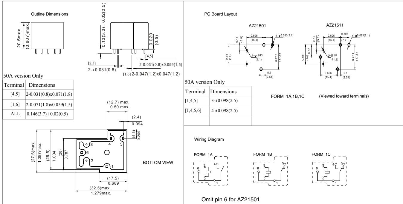
Dimensions in inches with metric equivalents in parentheses. Tolerance:  $\pm .010"$
