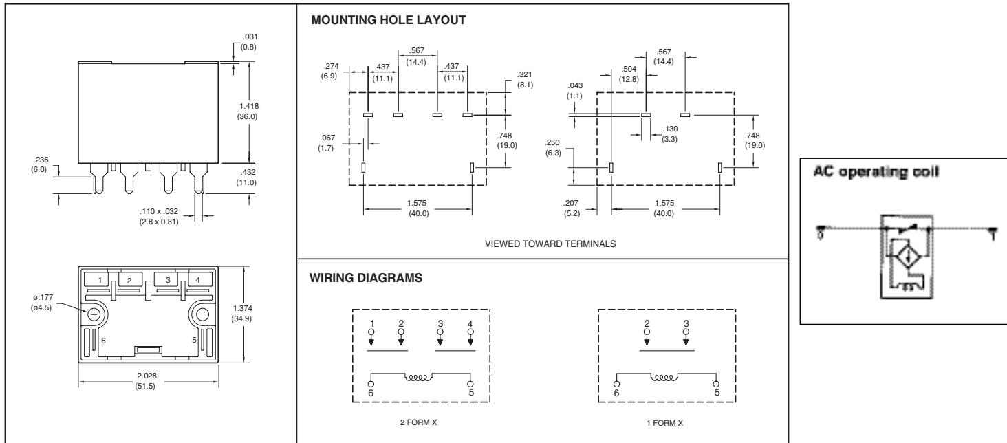
Dimensions in inches with metric equivalents in parentheses. Tolerance:  $\pm .010"$
