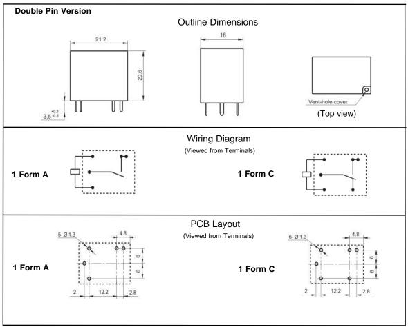
If no tolerance is shown, dimension <= 1mm tolerance is ±0.2mm;dimension > 1mm and <=5mm tolerance is ±0.3mm;dimension >5mm tolerance is ±0.4mm
