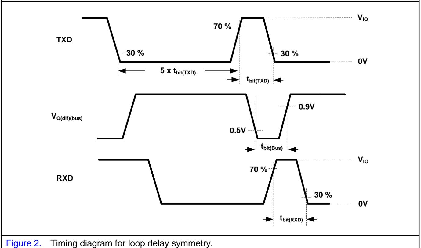
Figure 2. Timing diagram for loop delay symmetry.
