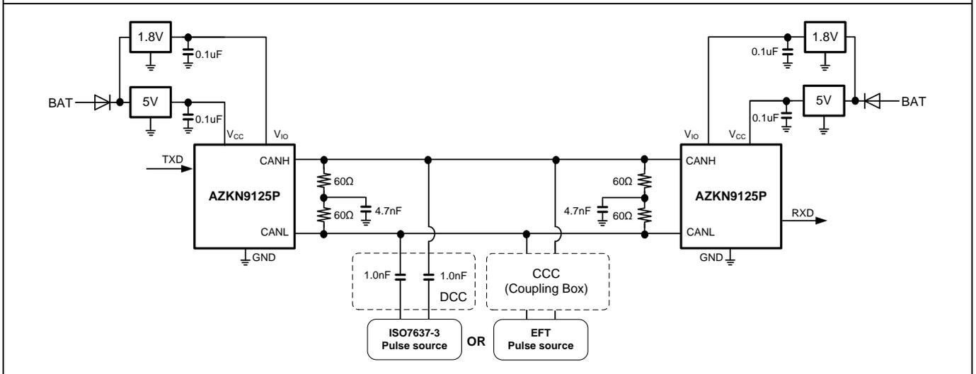
Figure 7. EFT coupling test circuit for AZKN9125P.
