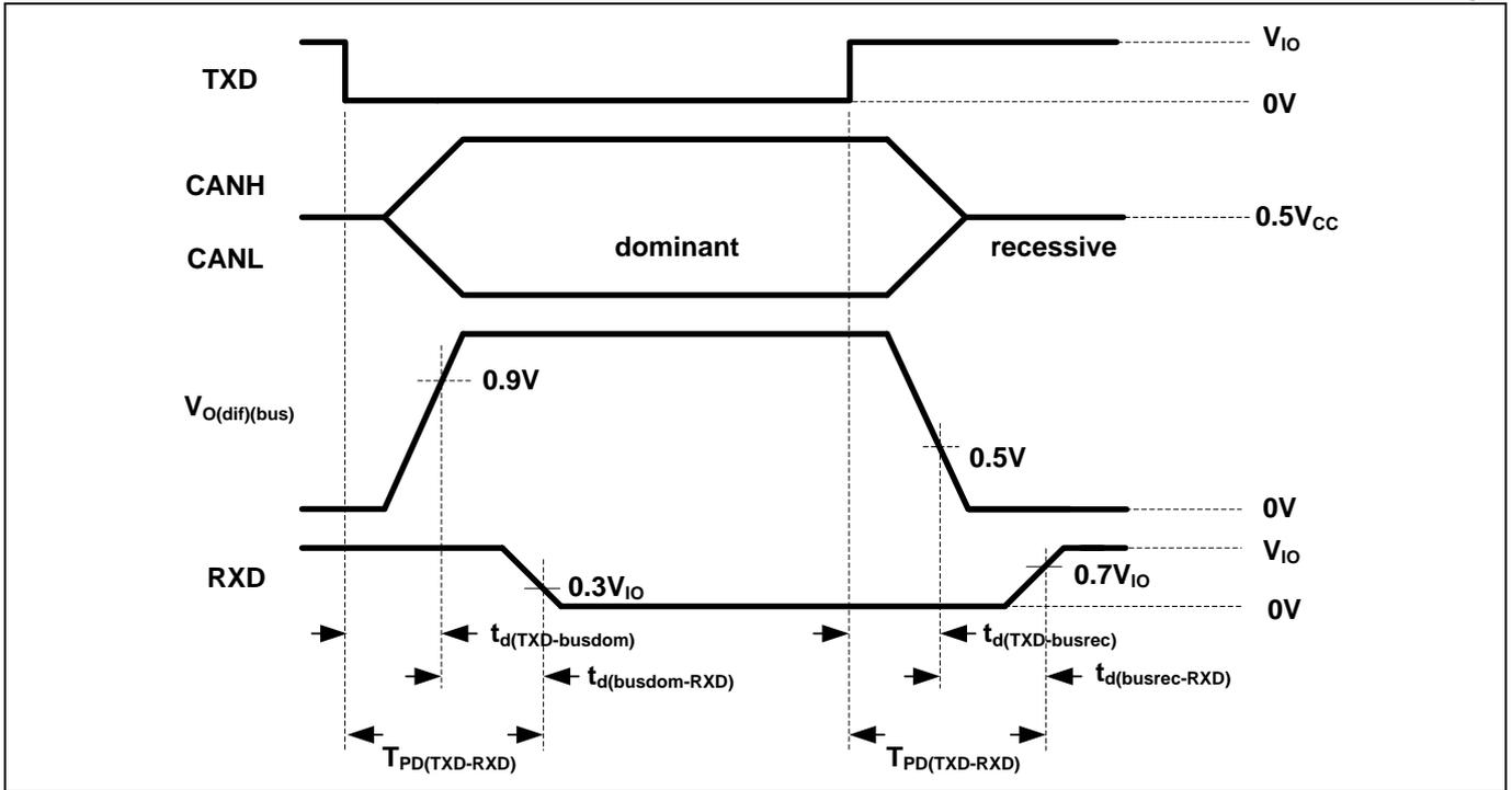
Figure 1. Timing diagram of the CAN transceiver.
