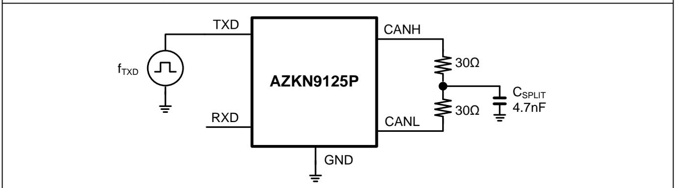
Figure 8. Test circuit for measuring transmitter driver symmetry.
