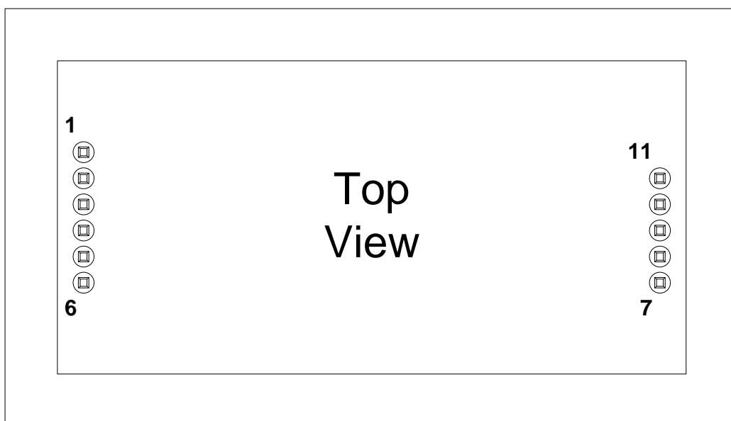
Figure 2: Ag5200 DIL Package Format
