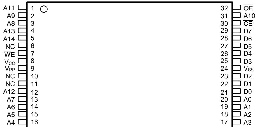
32-Pin — Standard Pinout
