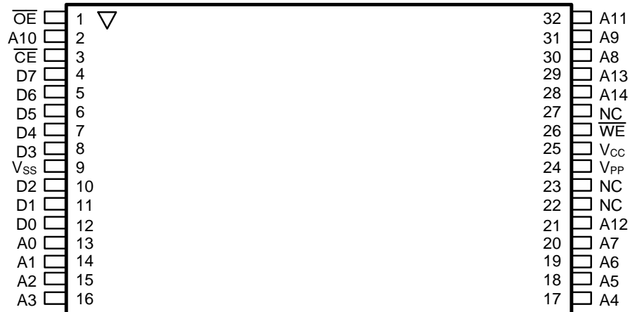
32-Pin — Reverse Pinout
