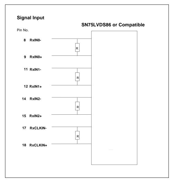
The module uses a 100ohm resistor between positive and negative data lines of each receiver input
