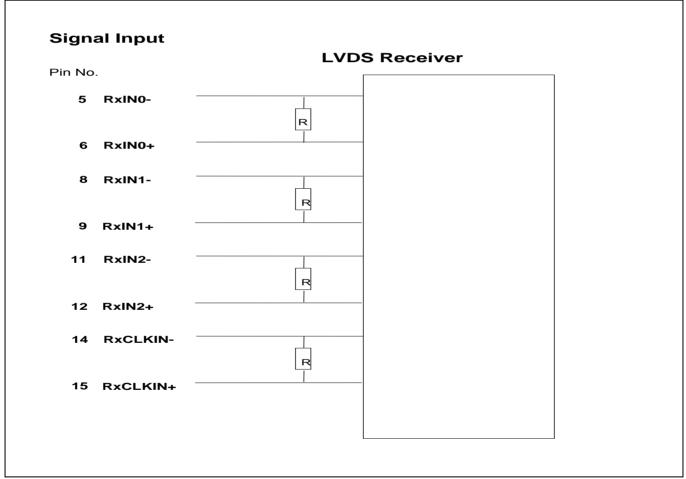
The module uses a 100ohm resistor between positive and negative data lines of each receiver input
