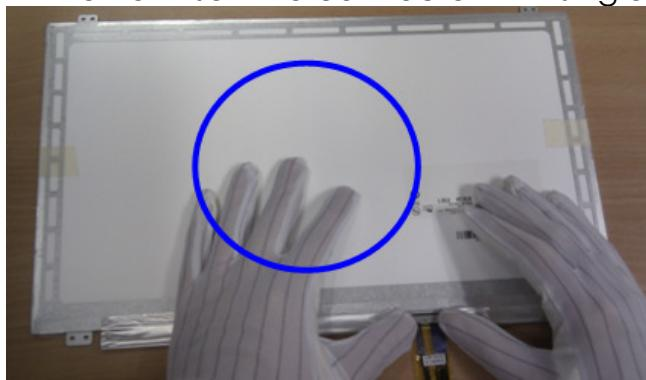
Insert the connector by pushing right and left edge.
