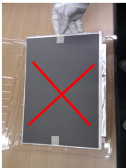
Do not lift and hold the panel with single hand at right or left side from tray.
