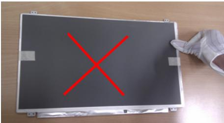
Do not press edge of panel to avoid glass broken.
