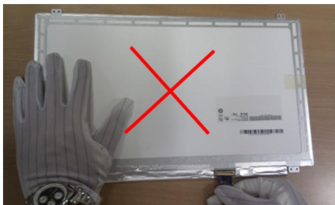
Do not insert the connector with single hand and touching the PCBA.
