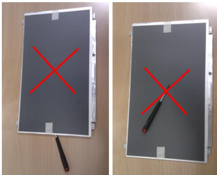
Do not put anything or tool on the panel to avoid the glass broken or polarizer scratch.
