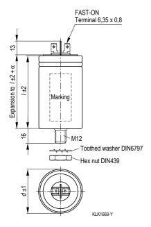
$\begin{array}{ll} \text{Creepage distance} & 10.0 \text{ mm} \\ \text{Clearance} & 16.5 \text{ mm} \\ \text{Diameter (Ø)} & 63.5 \text{ mm} \\ \text{Expansion } \alpha & \text{max. 12 mm} \\ \end{array}$
