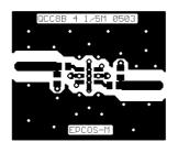
Optimised PCB layout for SAW filters in QCC8B package, pinning 1,5 (top side, scale 1:1)
