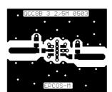
Optimised PCB layout for SAW filters in QCC8B package, pinning 1,5 (top side, scale 1:1)
