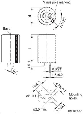
Large-size capacitors, snap-in version with 3 terminals (length (4.5 -1) mm.
