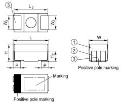
① Encapsulation: molded epoxy resin
