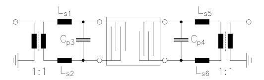
$$\begin{array}{l} L_{s1} = \ L_{s2} = \ 47 \ nH \\ L_{s5} = \ L_{s6} = \ 47 \ nH \\ C_{p3} = C_{p4} = \ 1,2 \ pF \end{array}$$
