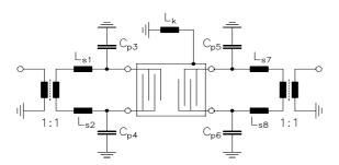
$$\begin{array}{l} L_{s1} = L_{s2} = 18 nH \\ C_{p3} = C_{p4} = 1,2 pF \\ C_{p5} = C_{p6} = 1,2 pF \\ L_{s7} = L_{s8} = 18 nH \\ L_{k} = 68 nH \end{array}$$
