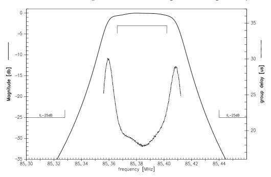
Normalized transfer function (wideband, measured single ended - single ended)
